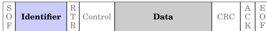
Fig. 1. Illustration of a CAN frame. The identifier is used for arbitration and, therefore, cannot be encrypted while the data might be encrypted. As a result, the identifier exposes information about the type of data to attackers due to the fixed coupling of identifiers and data in the automotive domain. The used acronyms are: SOF - Start of Frame, RTR - Remote Transmission Request, CRC - Cyclic Redundancy Check, ACK - Acknowledgment Slot, EOF - End of Frame.
